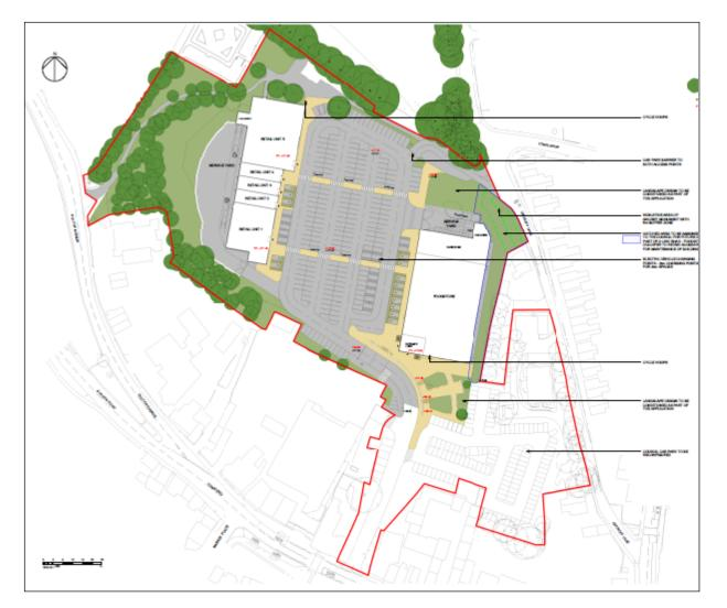
The main vehicular access to the site would be from Town End and a secondary access to the site would be provided on to Oxcroft Lane with each block having separate servicing configurations with service areas proposed to the rear of the retail terrace and to the side of
